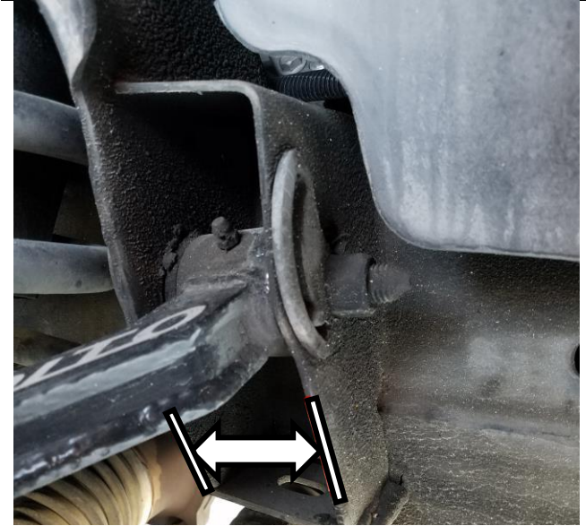
Figure 2: Factory Frame Service Perch Removal - After
