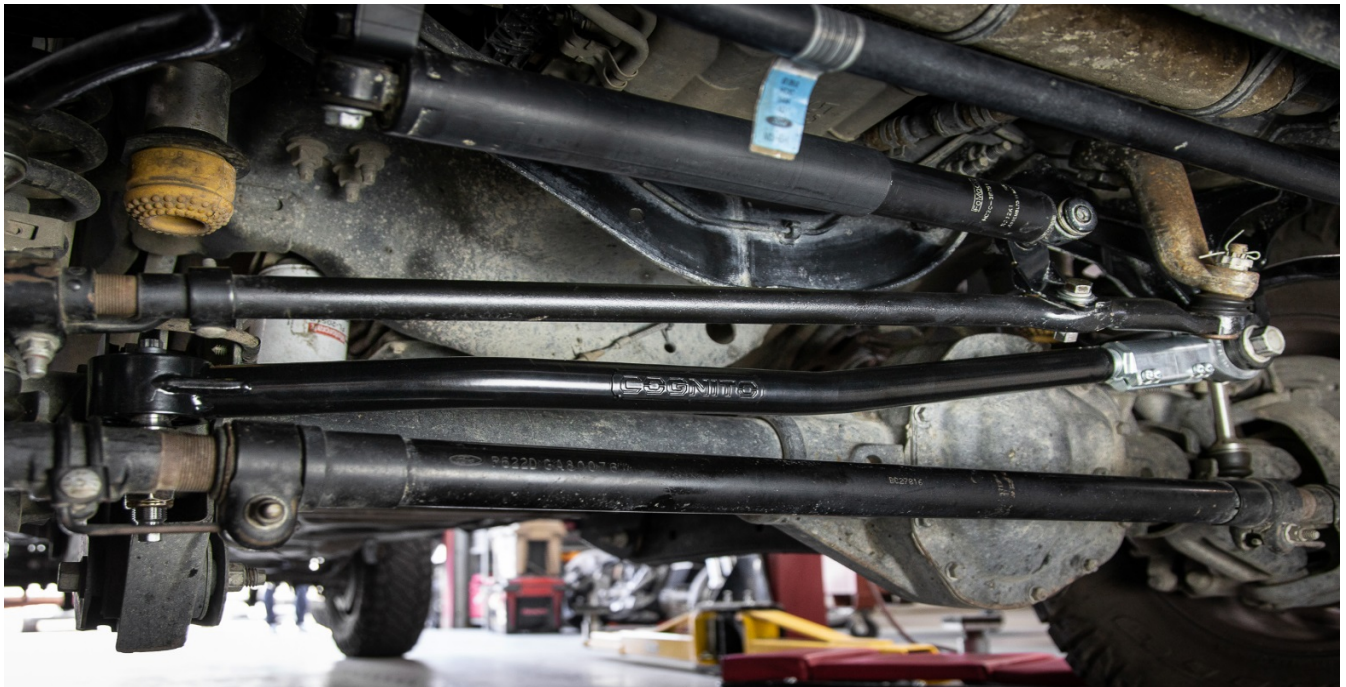
Figure 21: Installed Track Bar
