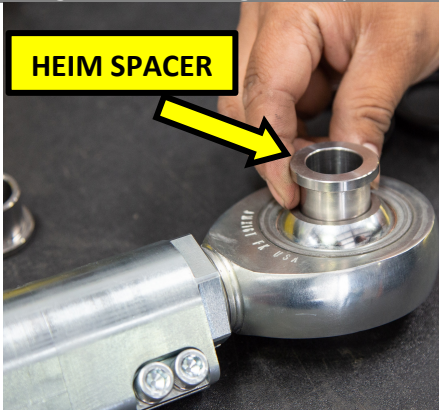
Figure 7: Installing Heim Spacer
