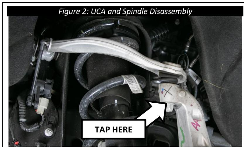
5. Remove the factory bolts and eccentric washers that connect the control arm to the frame and retain them for future use. Place them aside and note the order in which the components were removed, that way they may be re-installed in the same manner they came off.
