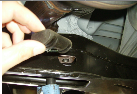
Figure 3: Remove Adjuster Nut
