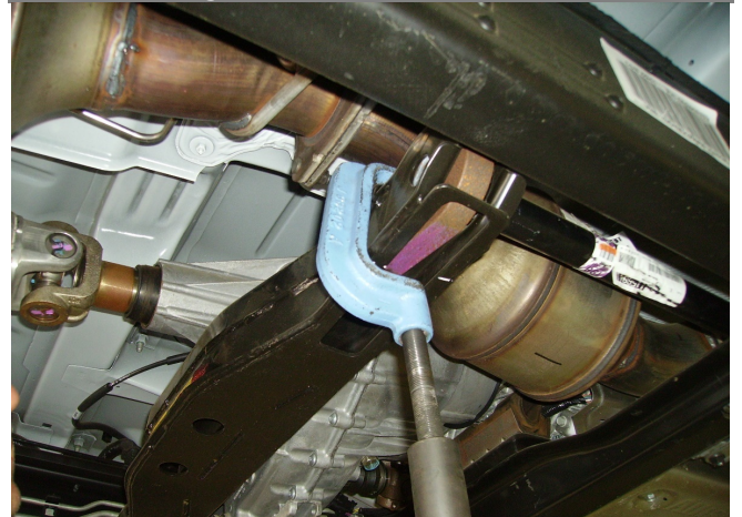
Figure 2: Unload Torsion Bar
