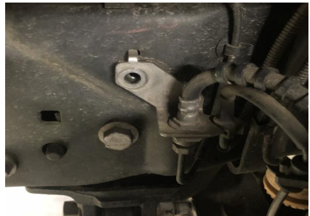
Figure 1B: OE Brake Line Bracket, Bolt Removed
