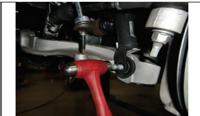
Gently tap lower strut mounting bolt out.
