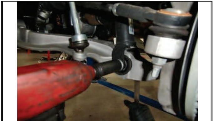
Remove lower strut mounting nut.
