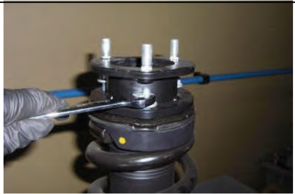
Attach new strut extension with OE hardware.
