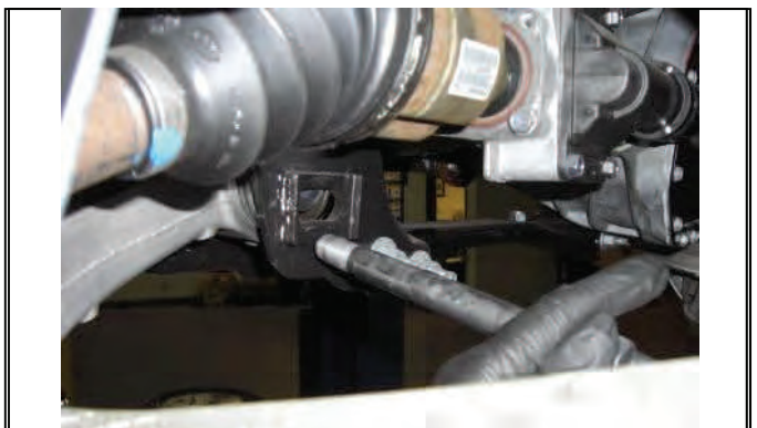
Remove lower control arm mounting bolts.
