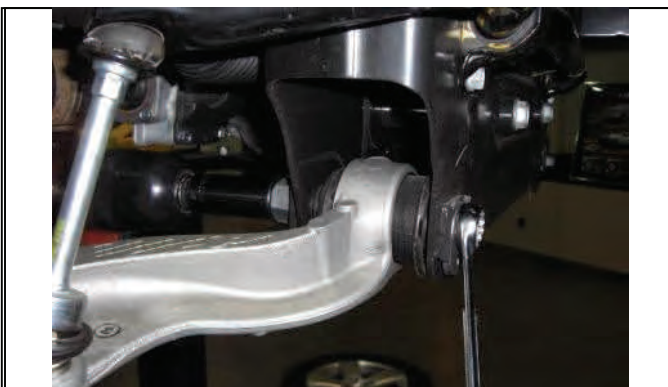
Loosen alignment cam nuts and bolts
