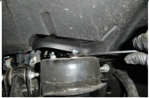
Now, remove upper strut mounting nuts.
