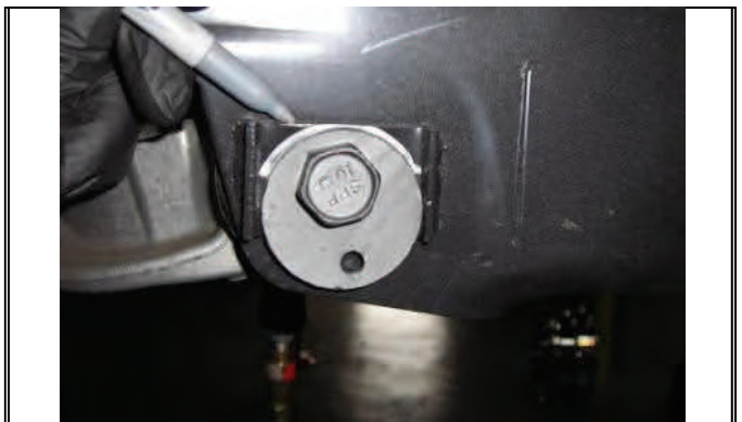
Mark front and rear lower control arm alignment cams.
