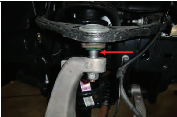
Picture shows separated upper ball joint. Note gap.
