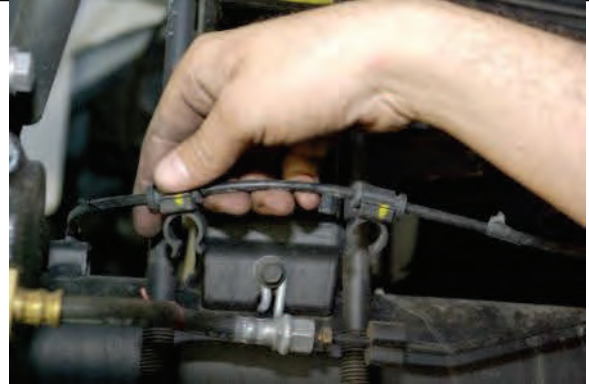
Vehicles with ABS/TC remove clips from U-bolts.
