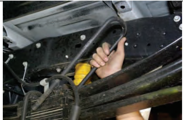
Remove U-bolts and slowly lower axle to remove OE block.
