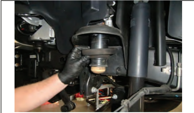
Remove the upper spring isolator to expose mounting hole
