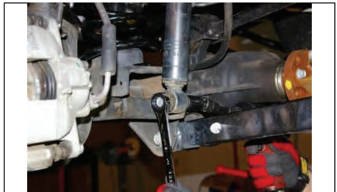
Reattach lower shock mount and tighten
