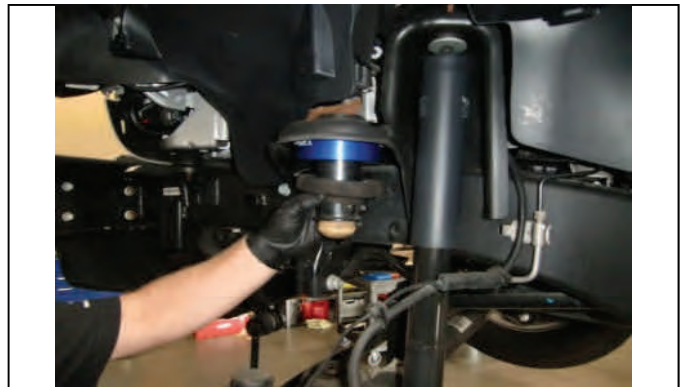
Tighten bolt and reinstall rubber isolator as shown
