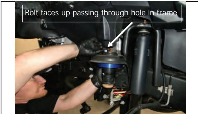
Attach spring spacer kit with provided hardware
