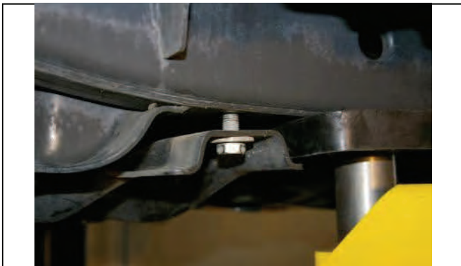
Loosen (2) front transfer case skid plate bolts.
