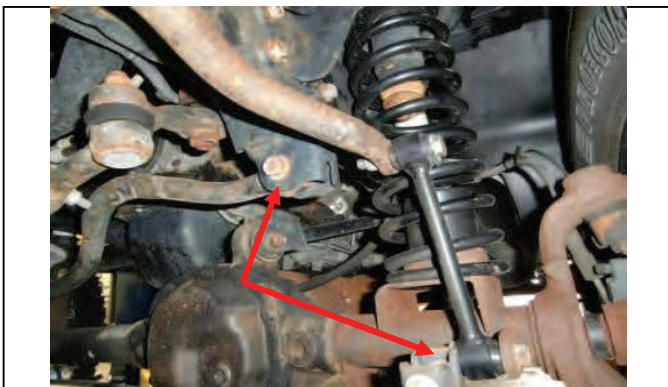
Reconnect lower swaybar endlinks and trac bar bolt
