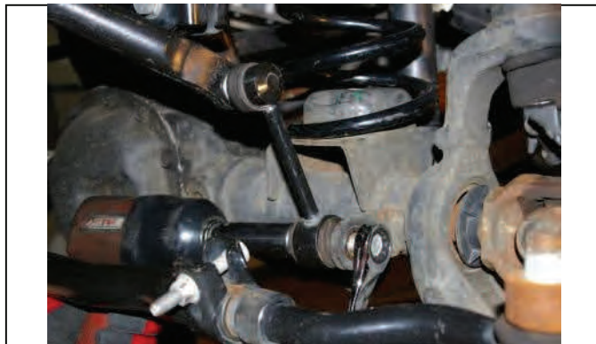
Disconnect dr./pass. lower front swaybar end links
