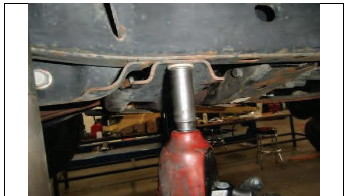
Tighten transfer case skid plate bolts, reinstall wheels
