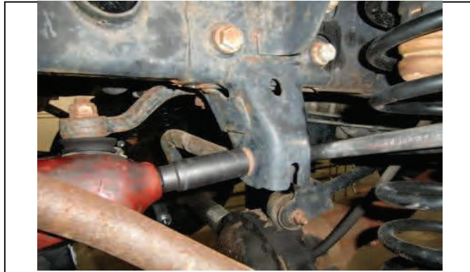
Support front axle and remove upper trac bar bolt.
