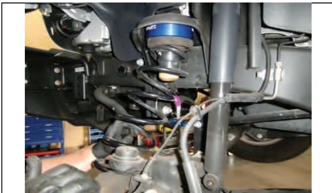
Reinstall coil spring in vehicle and raise axle
