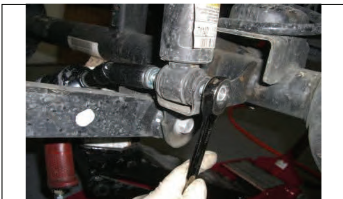
Disconnect and remove front lower shock hardware.
