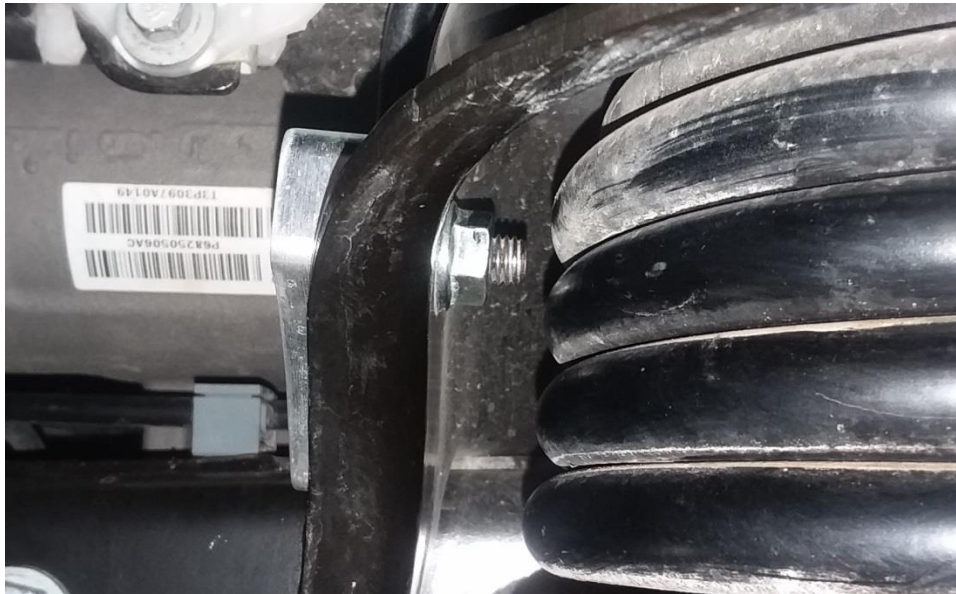
Figure 11 – Vehicle Left Side Serrated Flange Nut Installed
