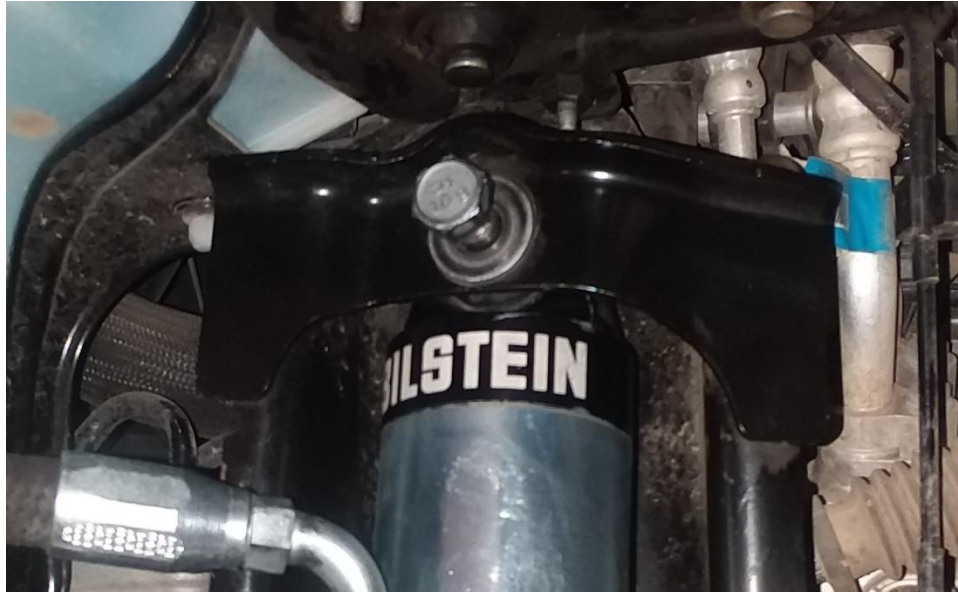
Figure 15 – Vehicle Left Side Upper Mount
