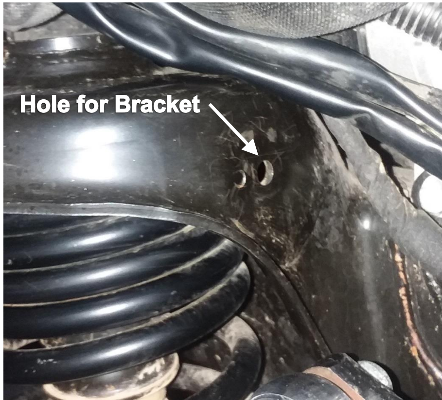
Figure 12 – Vehicle Right Side Spring Bucket
