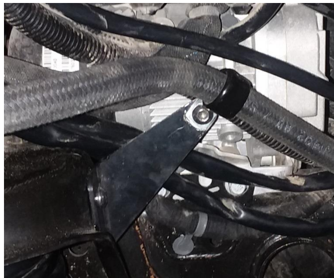
Figure 29 – Right Reservoir Hose Installed
