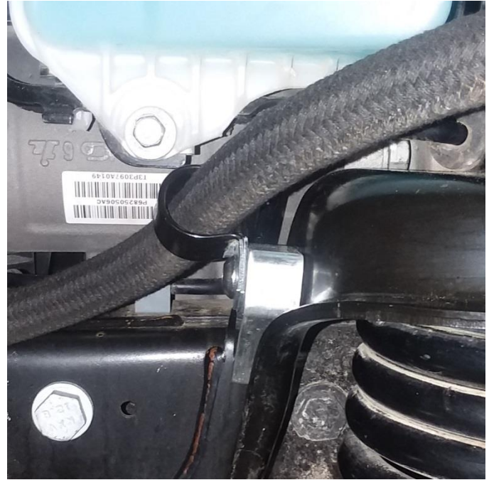
Figure 28 – Left Reservoir Hose Installed (Side View)
