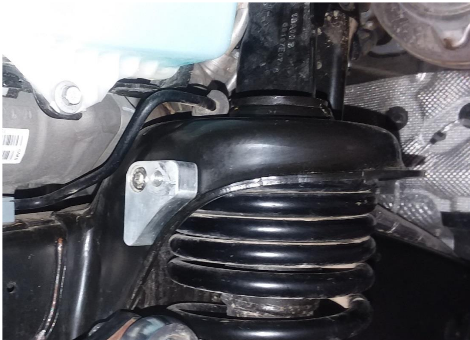
Figure 10 – Vehicle Left Side Reservoir Hose Mount Bracket
