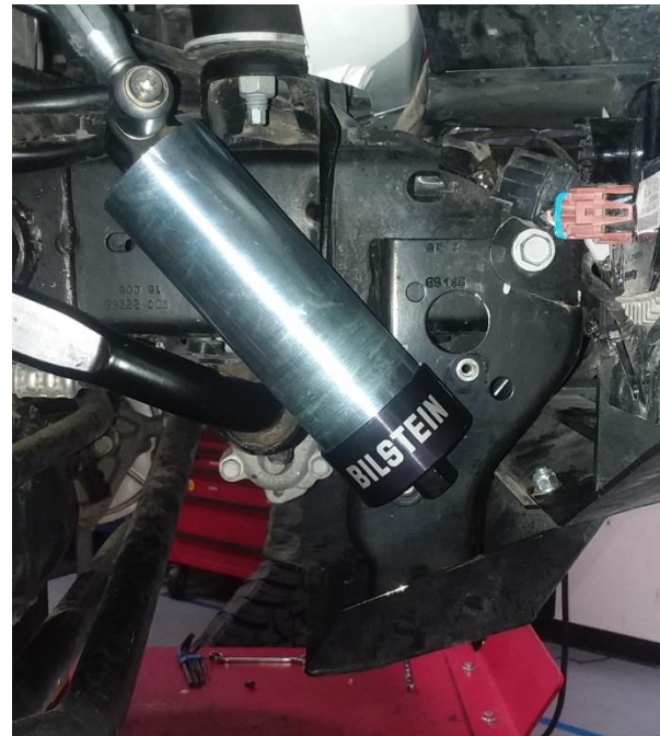
Figure 23 - Right Front Reservoir Slide Into Mount
