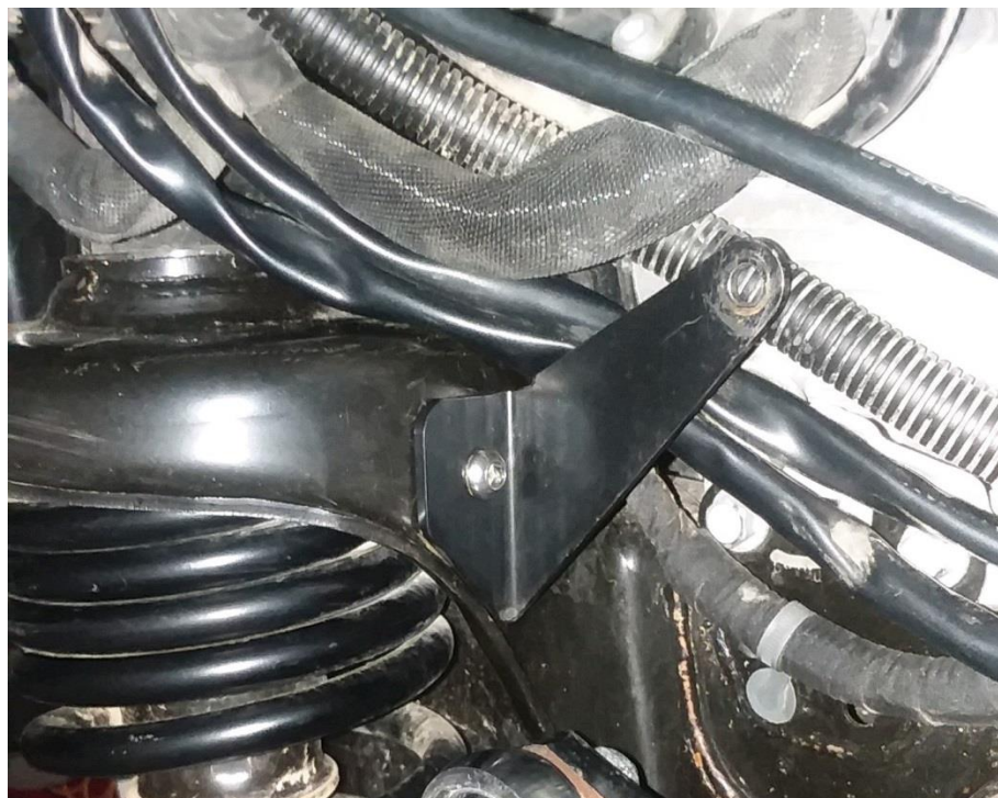
Figure 13 – Vehicle Right Side Hose Bracket
