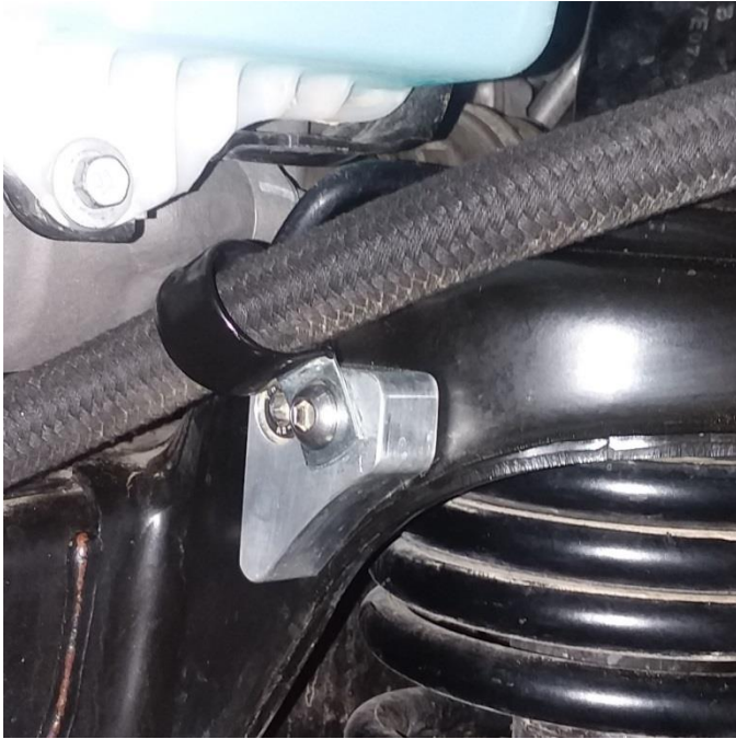
Figure 27 – Left Reservoir Hose Installed
