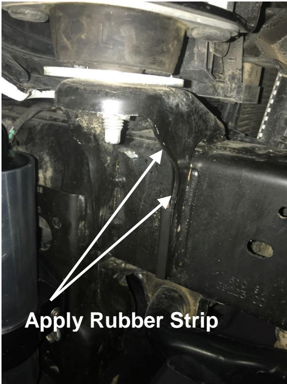
Figure 25 – Left Side Location for Rubber Strip
