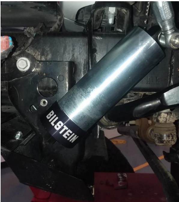
Figure 22 - Left Front Reservoir Slide Into Mount
