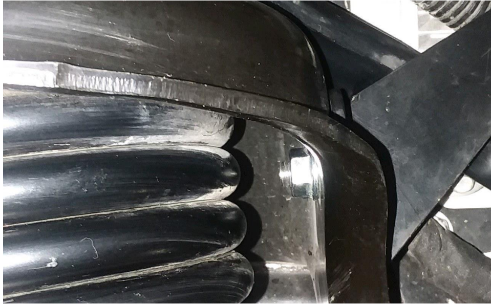
Figure 14 – Vehicle Right Side Serrated Flange Nut Installed
