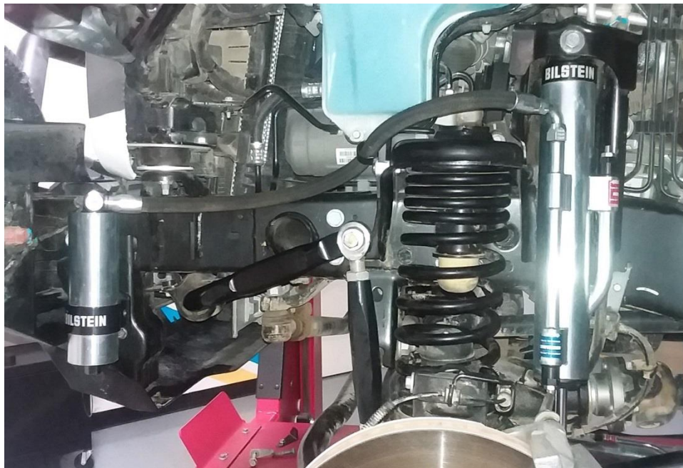
Left Side Installed (Without Inner Fender Liner)
