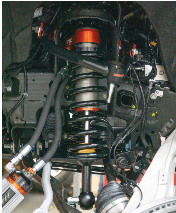
Fig. 13: Driver's side coil-over assembly is featured.
