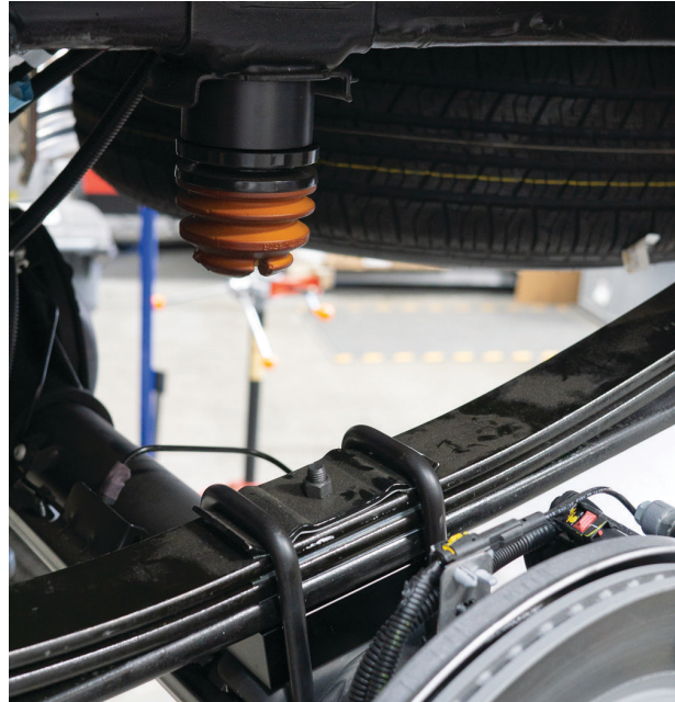
Fig. 26: Install the aftermarket lift block kit.
