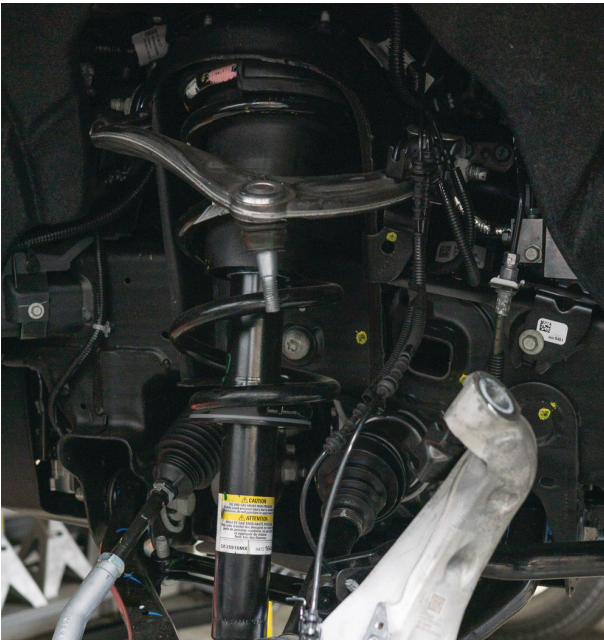
Fig. 5: Separate the UCA and upright.
