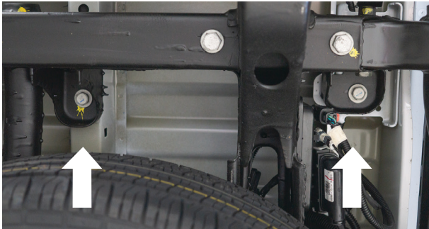
Fig. 30: Remove rear bed bolts (driver side shown).
