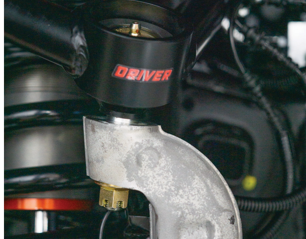
Fig. 18: Reattach UCA to the upright.
