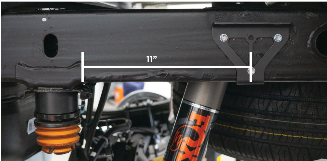
Fig. 37: Mount the reservoir bracket.
