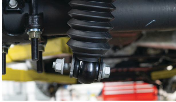
Fig. 35: Fasten the shock's lower mount.
