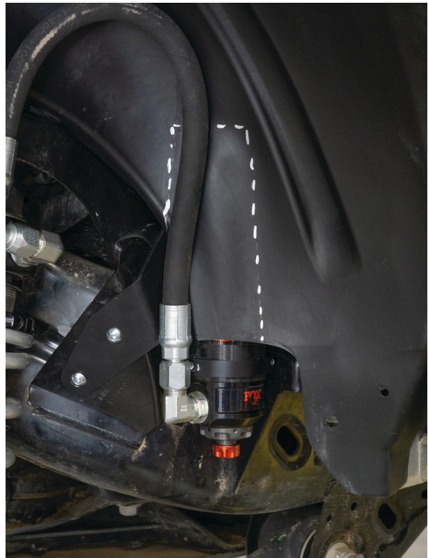
Fig. 36: Test fit the fender liner.
