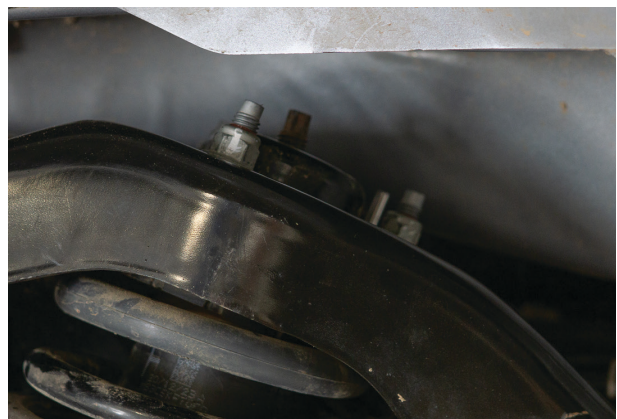
Fig. 27: Do not remove the center nut.
