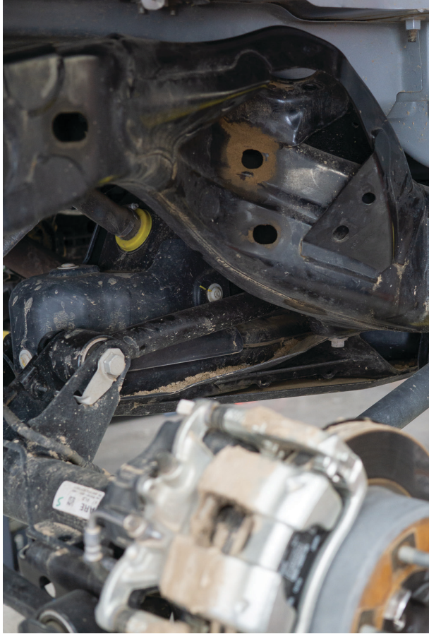
Fig. 28: Remove the stock coil-over.
