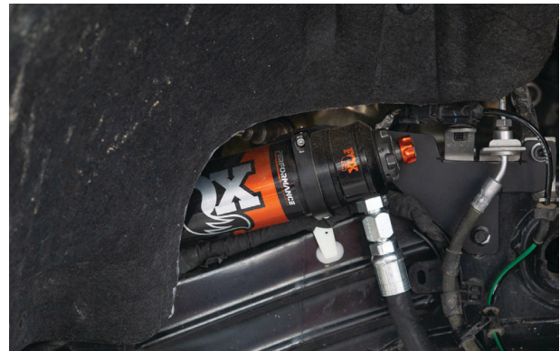
Fig. 23: Cut fender liner.
