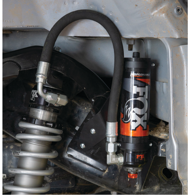
Fig. 34: Mount the reservoir to the mounting bracket.
