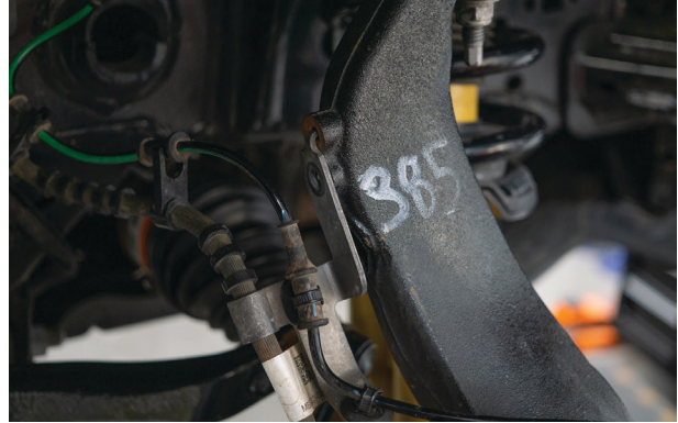
Fig. 4: Disconnect brake line bracket.
