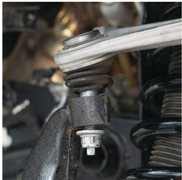
Fig. 8: Separate the UCA from the upright.
