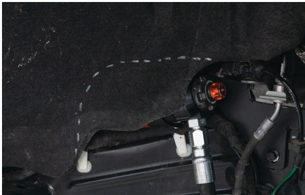
Fig. 22: Test fit the fender liner.
