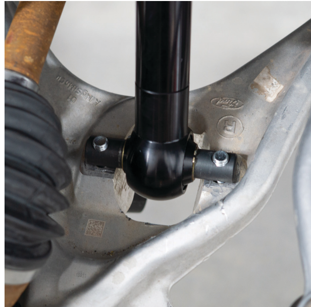
Fig. 15: Fasten the bar-pin bolts.
