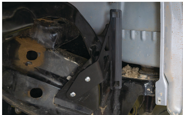
Fig. 31: Mount the reservoir bracket.
