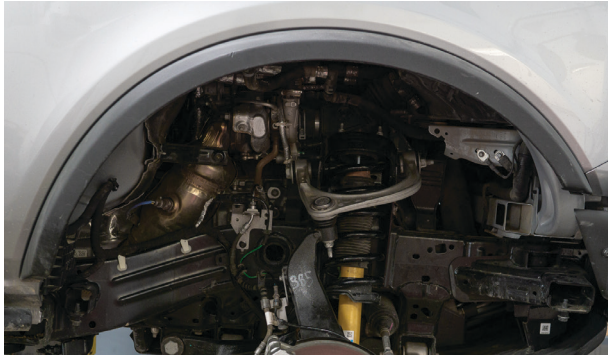
Fig. 1: Pull the fender liner.
