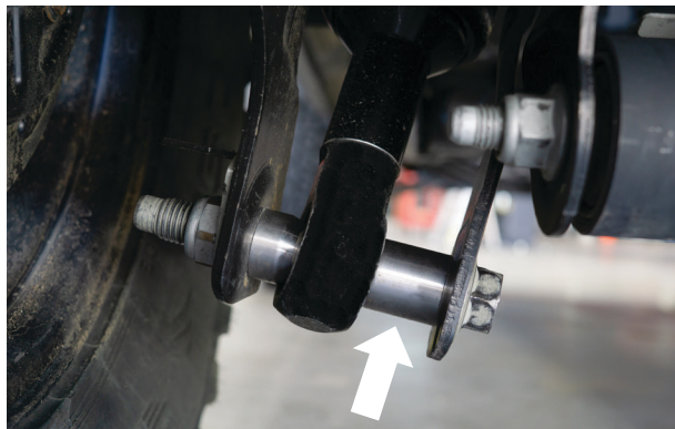
Fig. 34b: The larger spacer is mounted on the inboard side of the eyelet.
