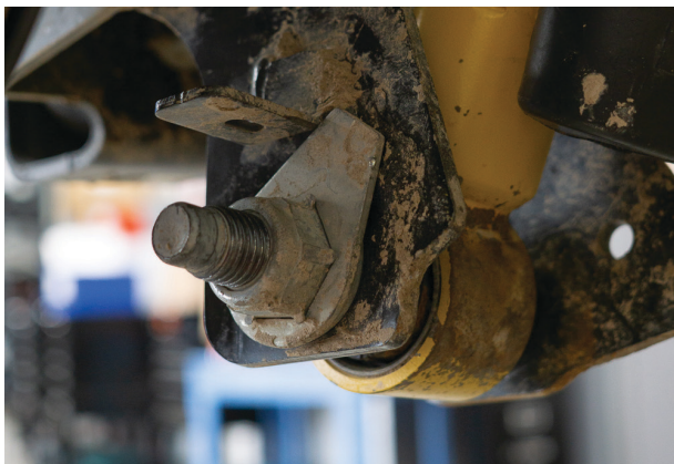
Fig. 26: Loosen the lower mounting bolt.
