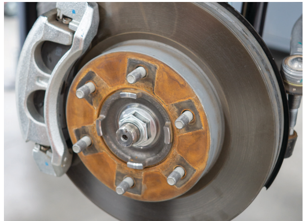
Fig. 18: Fasten the axle nut.
