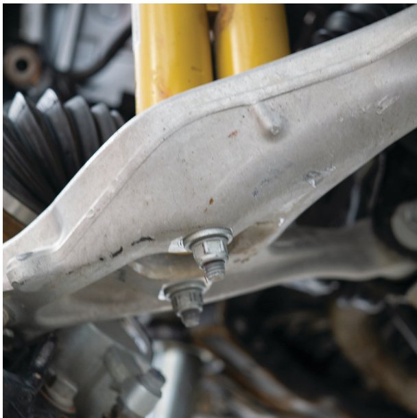
Fig. 11: Take off the bar-pin bolts.
