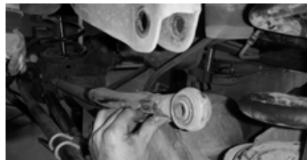
Fig. 1: Track bar removal
