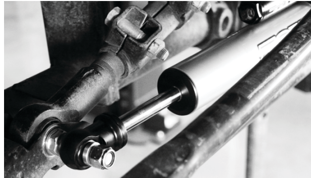
Fig. 3: Eyelet installed on track bar bolt.
