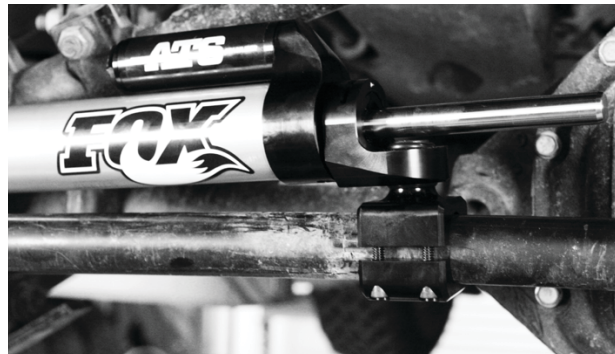
Fig. 4: Loosely clamp the stabilizer to the track bar.
