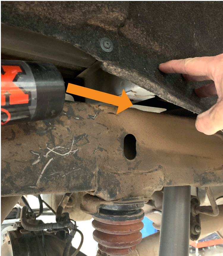
Figure 16: Bed is lifted \frac{3}{4} " on both sides of the vehicle just above the bump stop (70-inch bed shown).
