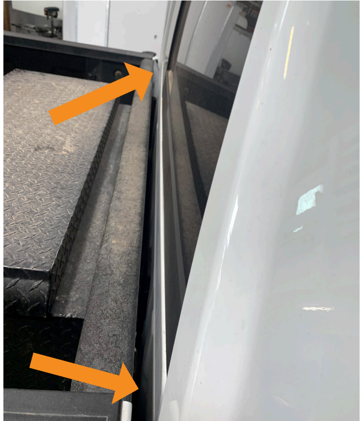
Figure 17: Rear of bed is raised \frac{3}{4} " on both sides of the vehicle and not touching the cab (70-inch bed shown).
