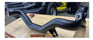
**13.** Using the provided clamps and turbo boot, install the Mishimoto hot-side intercooler pipe. Do not tighten the clamps, this will be done later. Reconnect the bypass valve hose and electrical harness.
