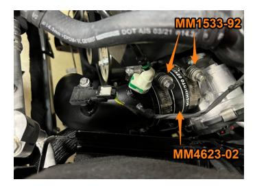
17. Install the intercooler adapters to both the inlet and outlet of the intercooler, then connect the Mishimoto hot and cold-side intercooler pipes to the intercooler adapters using the intercooler boots and provided clamps.
