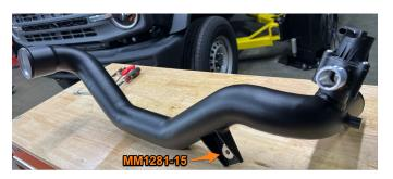
**16.** Using the provided clamps and turbo boot, install the Mishimoto hot-side intercooler pipe. Do not tighten the clamps, this will be done later. Reconnect the bypass valve hose and electrical harness. [MM4623-01, MM1533-66, and MM1533-79]
