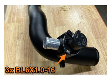
**15.** Install the provided grommet to the Mishimoto hot-side intercooler pipe. (MM1281-15)
