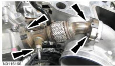
6. Release the clip and disconnect the CAC inlet tube from the turbocharger.
