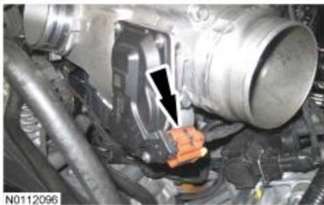
4. Disconnect the Exhaust Gas Recirculation Temperature (EGRT) sensor electrical connector and the wire harness retainer.
