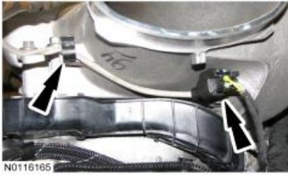
5. Remove the 4 bolts and the EGR bypass outlet pipe.
