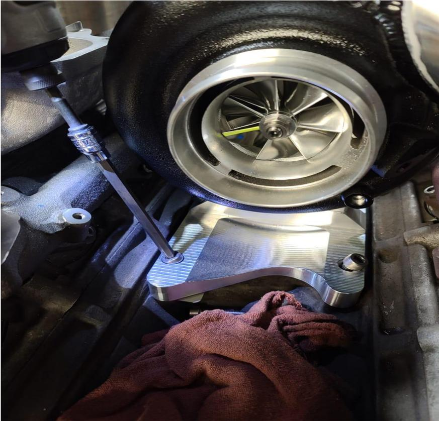
**4. Torque Turbocharger To Factory Recommendation**
