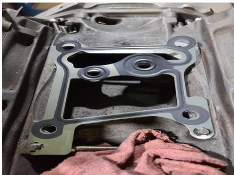
**NOTE: ENGINE MUST HAVE DOWEL PINS TO LOCATE TURBO PROPERLY WITH OIL FEED HOLE FAILURE TO DO SO MAY VOID WARRANTY OF TURBO**
