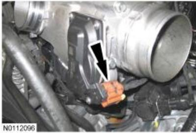
8. Connect the CAC outlet tube to the TB and install the clip.
