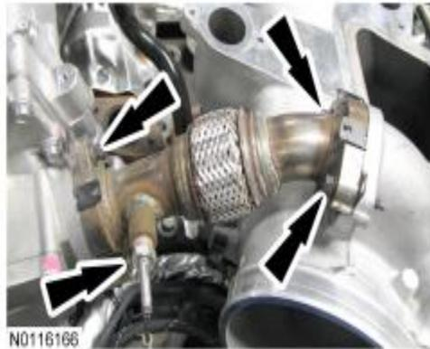
6. Connect the EGRT sensor electrical connector and the wire harness retainer.
